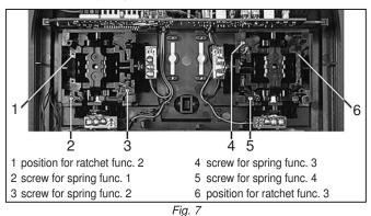
The position of the throttle ratchet on each stick is shown in Fig. 7.
