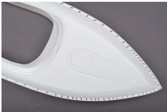
Fig. adhesive surface in the deck edge
