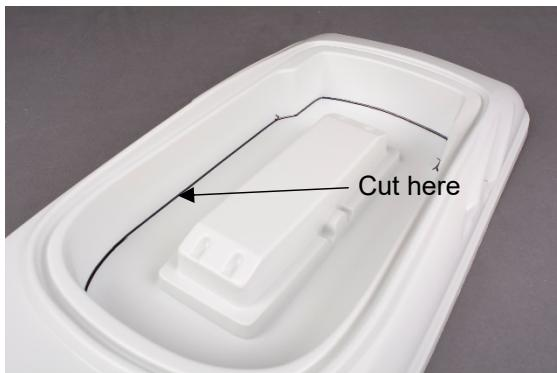
Fig. Cut off inner area
