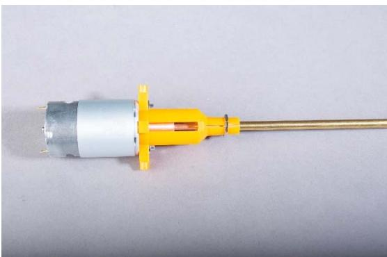
Fig. coupling flange fixed and sterntube inserted
