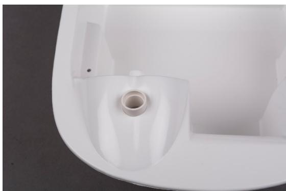
Fig. compass housing glued in
