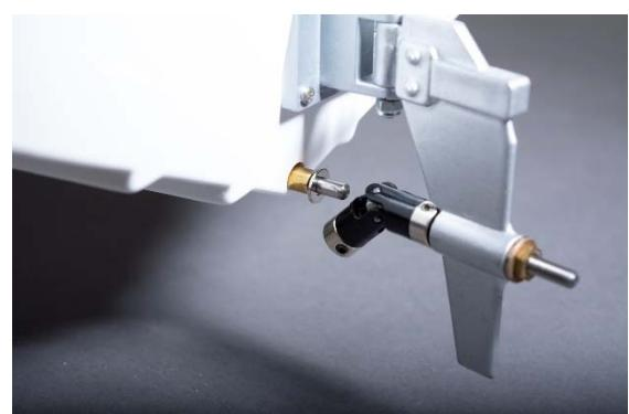
Fig. sterntube placed with washer
