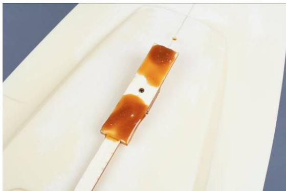
Coat the upper side of board 1.2 with Stabilit-Express. Insert the board with the handle into the hull and screw the eye bolt 1.6 through the deck from above to secure and tighten. Clamp the handle to the edge of the sliding hatch until the adhesive has cured. Make sure that no glue gets to the screw thread, otherwise the eyebolt is stuck and cannot be loosened any more. After the adhesive has dried, break off the handle at the predetermined breaking points.
