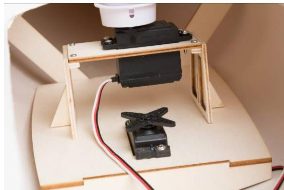
Fig. Sail winch frame on RC board
