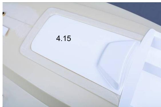
Fig. fitting the sliding hatch
