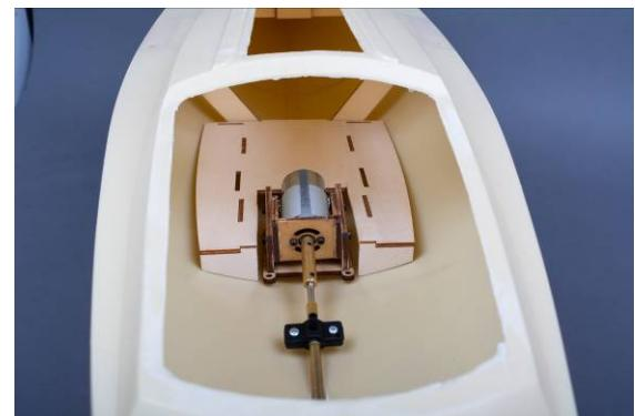
Fig. Placing the drive in the hull
