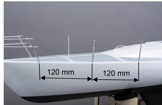
Fig. Installing railing stanchions
