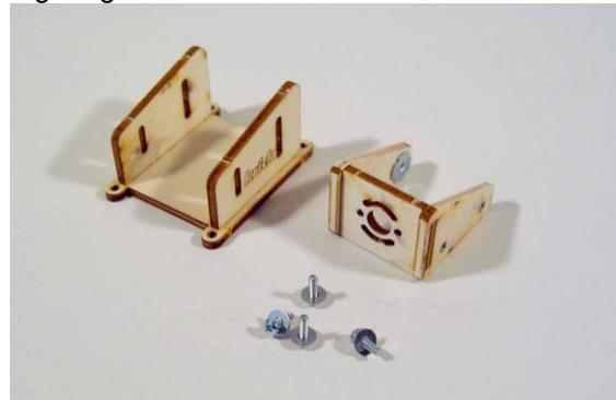
Fig. Motor mount glued
