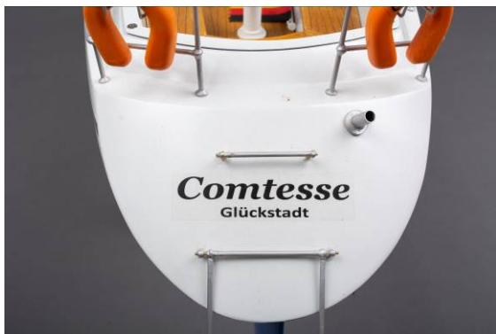
Fig. bathing ladder folded down, additional rung
