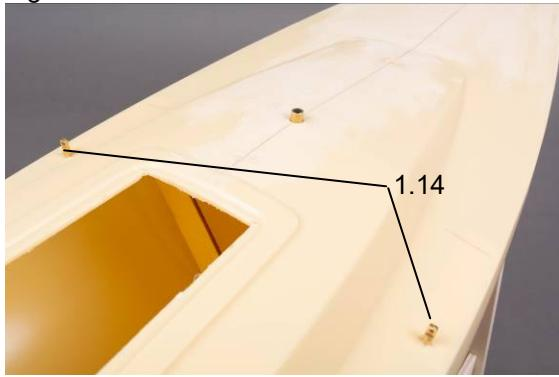
Now push the reinforcement plates for the shroud fastening into the slots in the frame and check the position by screwing in the eyebolts, part 1.14.
