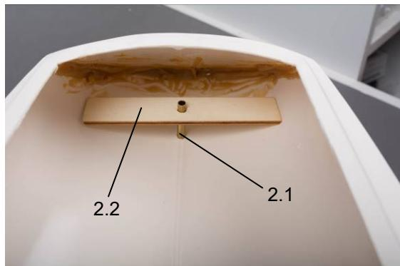
Insert the rudder from below and align it. Align the rudder so that it is exactly aligned with the keel when viewed from behind. When viewed from the side, align the rudder so that it is evenly spaced from the hull over its entire width. The rudder must be freely rotatable in both directions of rotation.
