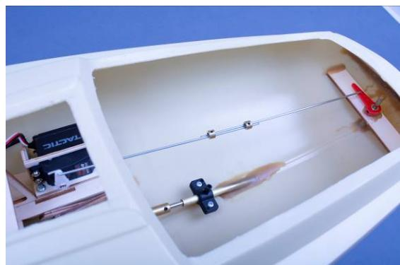
Fig. connection servo and rudder
