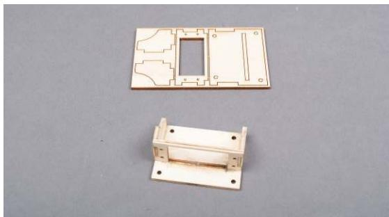
Fig. laser board and finished servo mount
