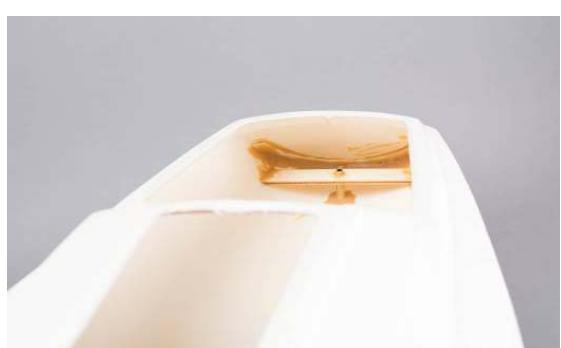
Fig. glued rudder bearing
