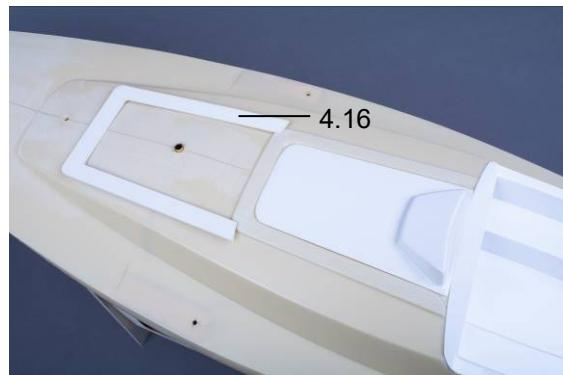
Fig. sliding hatch and frame
