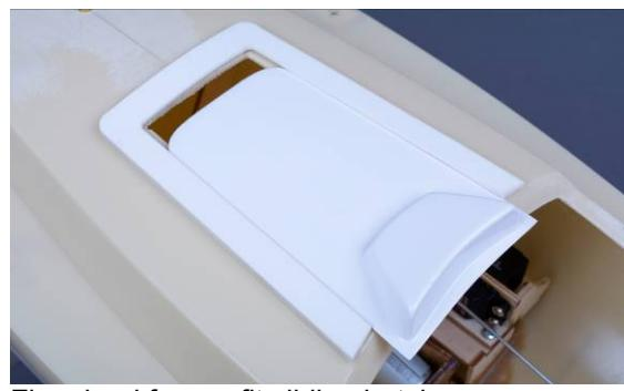
Fig. glued frame, fit sliding hatch
