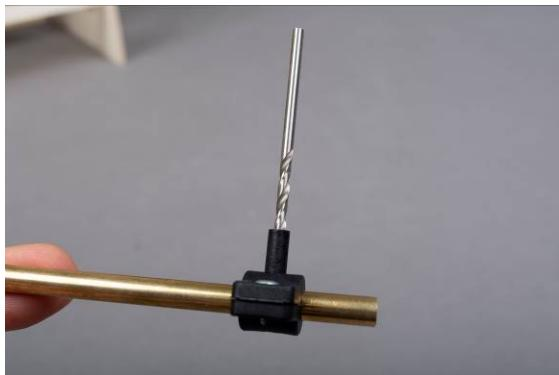
Abb Fig. Drill lubrication hole in sterntube
