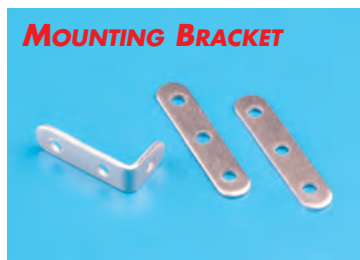
MOUNTING BRACKET Made of aluminum for attaching to masts and booms with 2 screws. The second end with free bore can be angled angular or vertically, be used to attach a leash, shroud or stay. Dimension 5 x 25 mm, holes 2 mm
