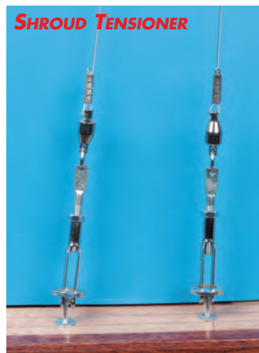
SHROUD TENSIONER Turnbuckle with swivel, eye bolts at top and bottom, clevis and nut. For easy adjustment of the shroud or stay length. Thread M3, total length approx. 70 mm
