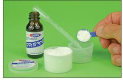
10 Mixed in equal parts the pipette is used to transfer a measured quantity of the liquid to the mixing container while the catalyst powder is metered out with the plastic measure. Increasing the powder content will not only result in a faster cure time but will also change the consistency to a syrupy solution.
