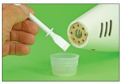
Mix the glue for some 5 or 10 minutes before you're ready to apply it. Once the glue has been applied you must avoid moving the joint until it has properly cured – a period of 30 to 40 minutes.
