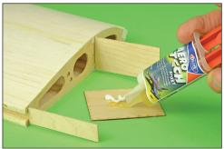
Aero Tech is supplied in a syringe dispenser that, crucially, allows equal quantities of both parts to be squeezed onto a mixing board at the same time.
