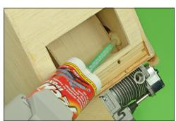
The dispenser with its disposable mixing nozzles allows you to deposit a correctly mixed quantity of epoxy in the most difficult of places i.e. behind a bulkhead or fire wall.
