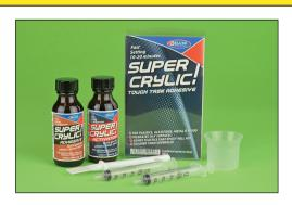
This high-tech, two part, very high strength glue forms a flexible joint in plastics, glass fibre, metal, and wood. Once cured it's tougher than superglue and will bond the plastics that epoxy struggles with. Super Crylic also tolerates oily surfaces, but is not suitable for expanded polystyrene, Depron or blue foam.
