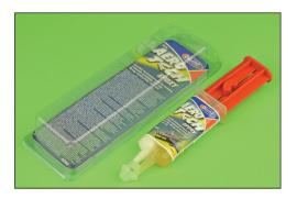
Aero Tech is a non-dip epoxy resin that will bond previously cured epoxy, GRP, carbon fibre, aluminium alloy, ply, and hardwood. The mixed glue will gel in three to four hours and sets in 24 hours.
