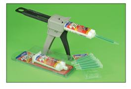
The Aero Tech dispenser gun uses the same glue that's in the syringe dispenser although the tube is of a different design (in order to fit the gun) and has disposable nozzles that, cleverly, mixes the two components as the gun's trigger is squeezed.
