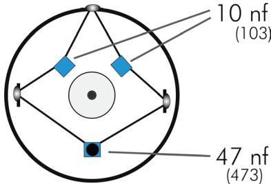
**Note:** The interference suppression kit minimizes interference from the electric motor to the controller and the RC receiver system. It should be used for all applications.
