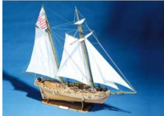
The revenue cutter Alert was used at the coasts of the United States for pursuit by smugglers. For this reason it was equipped with large sails and a wedge-shaped deep keel around faster and more highly at the wind sails. In the ship center at deck the Alert is equipped with a swivelling Kannonade with all accessories, which gives a very beautiful historical idea of the work at that time on board.
