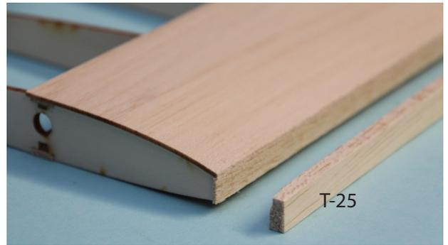
7.13 After the glue has cured, the wing can be removed from the building board. The leading edge is now sanded according to the course of the profile. Make sure that the leading edge is sanded really evenly and straight, not wavy or crooked.
